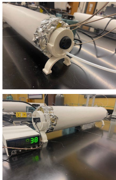
Figure1: Homemade speed of sound tube.
