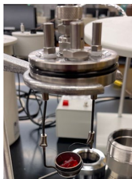
Figure 3: Bomb calorimetry set up with gummy bear sample
