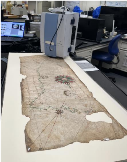
Image 4: The portable FTIR setup for analysis of the Portolan chart.
